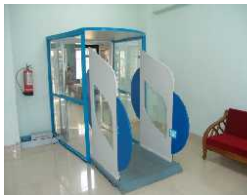
THE RADIO-FREQUENCY IDENTIFICATION DETECTION-CAPABLE SECURITY GATE AT THE ENTRANCE TO THE LIBRARY RECEPTION COUNTER
